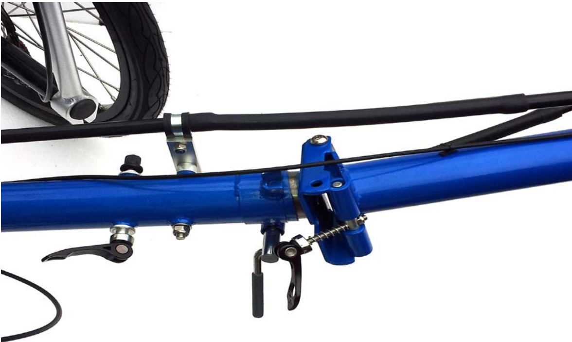
Step 1: Release the lever, rotate the frame, open the hinge.
