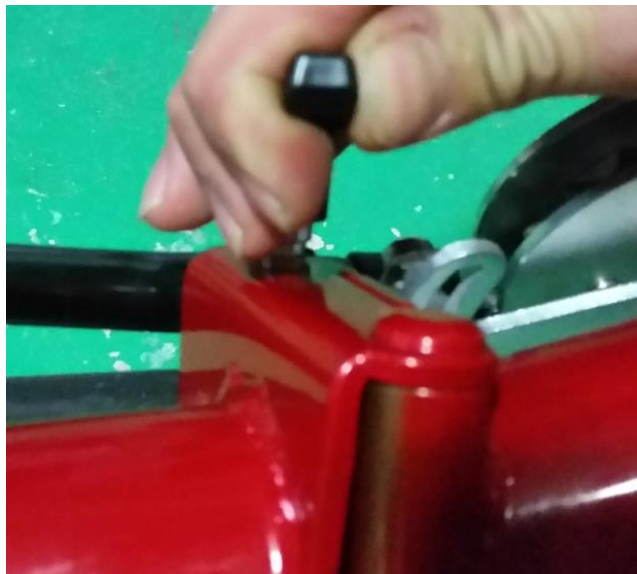
Step 5: Rotate the lever counter-clockwise until it is tight enough
