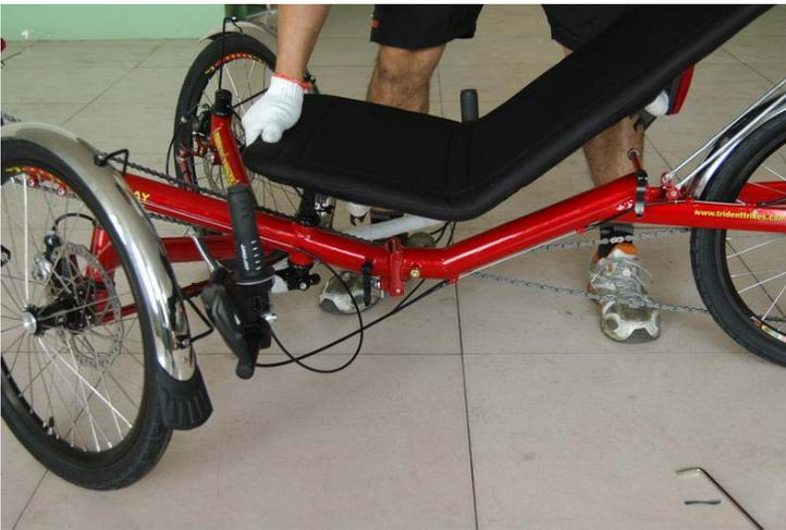
Loosen the quick release lever that holds the folding hinge and let it hang straight downward.
