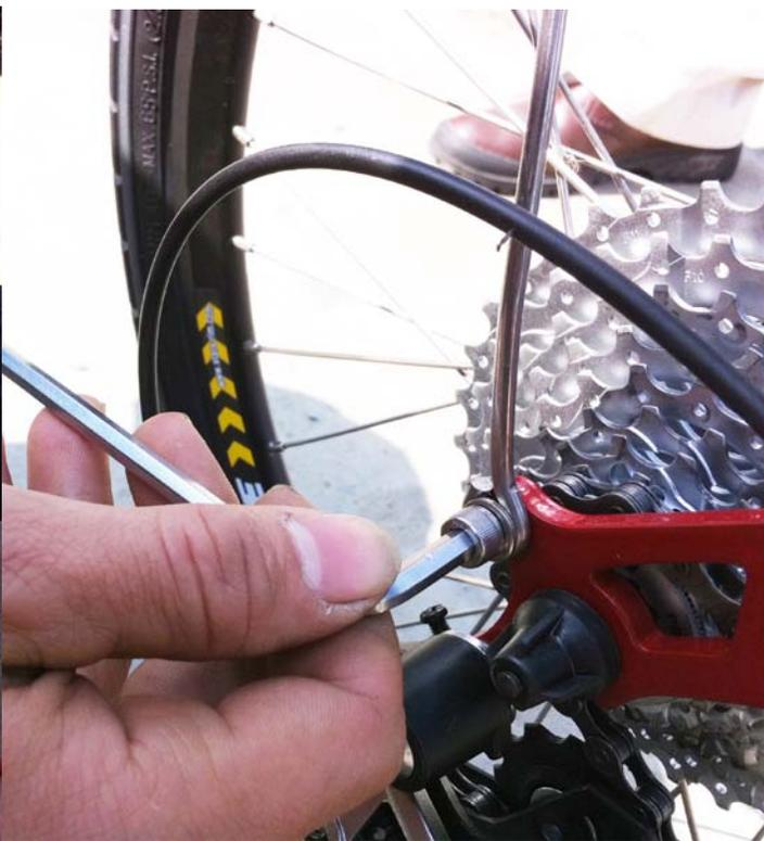
The rear rack gets attached by means of 2 rods that go from the rack to the frame support as well as 2 bolts/washer/nuts that attach to the holes in the dropouts. Please refer to the following pictures.
