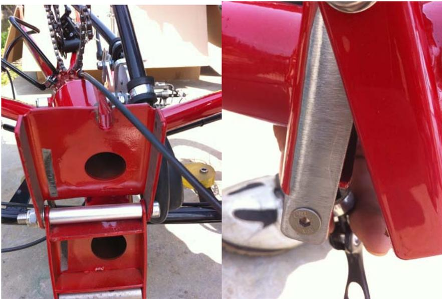
**Step 2:** To prevent shipping damage, the rear derailleur is not attached to the frame. Using an allen wrench, attach the rear derailleur as shown in the picture. Then attach the rear wheel to the trike and tighten the quick release.
