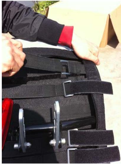
**Step 3:** Fasten the seat to the frame using the provided quick release skewers. It is easiest to do the bottom first. You have a choice of 3 seat heights . On the top you have four angle choices. Most people prefer to start with the more upright of the positions. Tighten quick release skewers fully.
