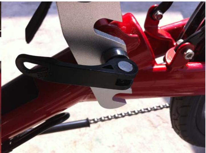
**Step 4:** Adjust boom length. The Boom is shipped turned at a 90 Degree angle. Loosen the boom and make sure the dreailleir post is perpendicular to the ground . Tighten a little so the boom does not rotate and attach the pedals - remember that the left pedal has reverse threads. Loosen boom bolts FULLY using a 6MM Hex Wrench. . Note: it is always important to fully loosen screws when adjusting boom- otherwise you will severely scratch the finish. It is also helpful if you put a
