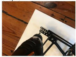
**Step 3**: Remove the seat from your trike and then remove both bolts from either side of the Black Rear Seat Mount on the frame using a 6 mm Allen Wrench. You can also remove the flag holder from the left side as you will no longer need it- the rack has a built in flag holder.
