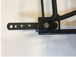
**Step 2**: Drill the hole at the bottom slightly larger than it is originally. It needs to be 8mm or 5/16"
