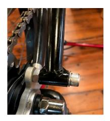
**Step 4**: Remove the 8 mm nut that was in between the Black Rear Seat Mount and the frame. And replace it with an 8 mm Washer on both sides.
