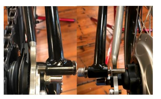
**Step 5**: Put the rack on the protruding bolt and screw back into the frame- do not tighten until both sides are in. Once they are in you can tighten fully, The left side also gets the nut on the inside of the frame that you removed when you took out the flag holder.
