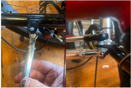
Step 3: Place the clamp that has a tie rod end and about 1" from the end of the cylinder on the steering damper. Put the M8 x 40mm Bolt from the back of the tie rod and put 2 8 mm nuts on this bolt. Screw the 8mm bolt onto 1 side of the tube clamp. Cut the rubber strip to fit the Trike Tubing, peel the paper off, and the place the rubber strip on the tube opposite of the bolt.
