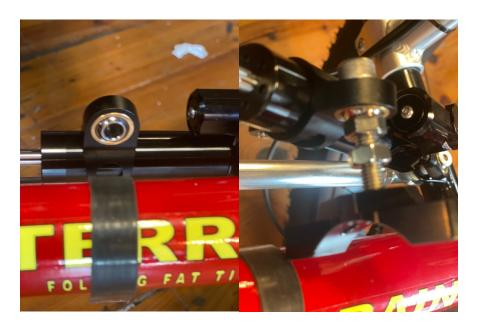
Step 4: Using the included M6 x 40 Bolts , Attach both sides of the clamp over the rubber piece on the frame tube. At this point you can fully tighten all the bolts. You can adjust how much damper you want using the knob on top of the steering damper.
